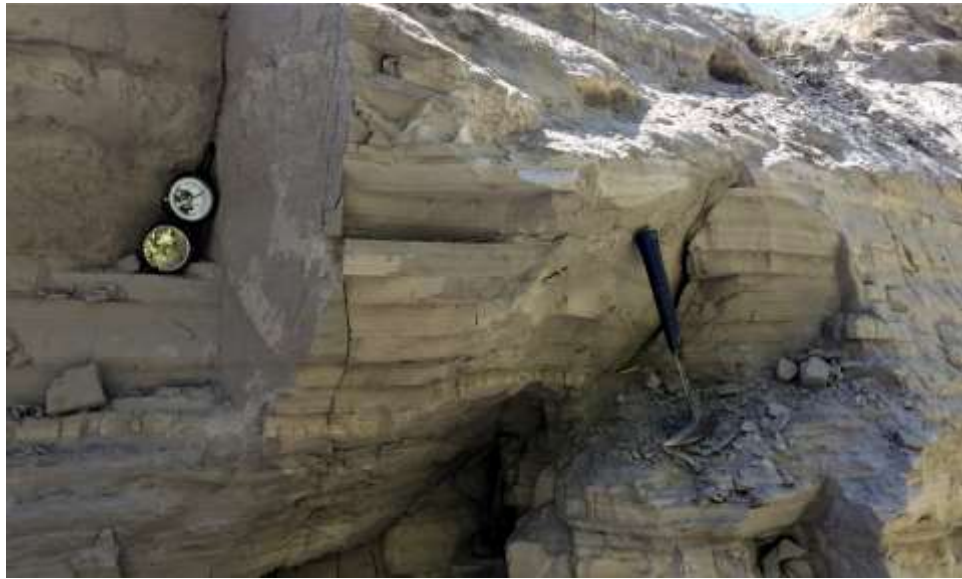
Photo 4-35 View of Vertical and Oblique Joints in Clayey Silt at Sarat Village.
