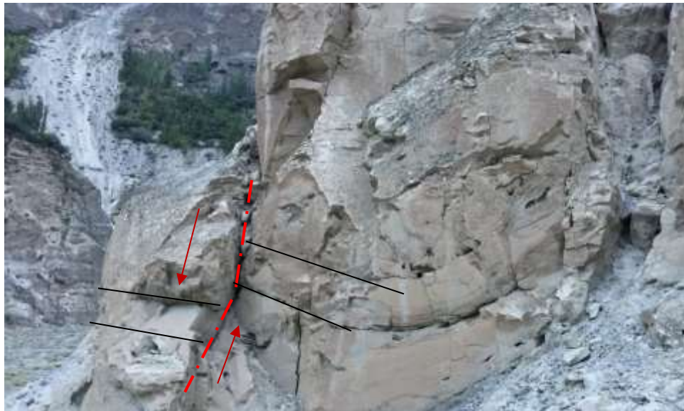
Photo 4-65 View of Micro Fault and Displacement of Blocks.
