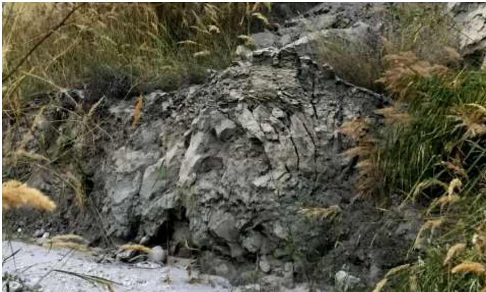
Photo 4-38 Folded and Sheared Clayey Silt at Sarat Village.
