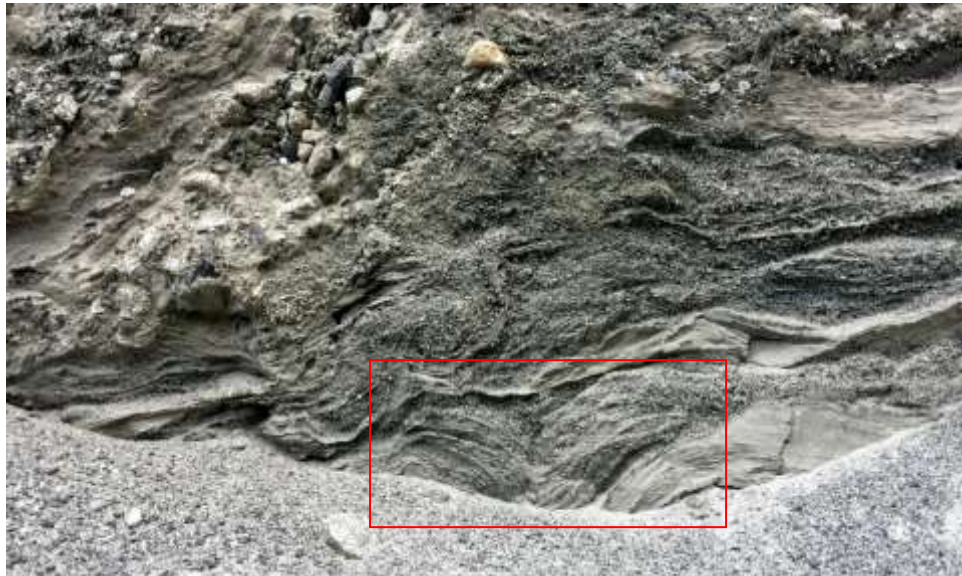
Photo 4-27 Folding in RBGM and Sand Beds.
